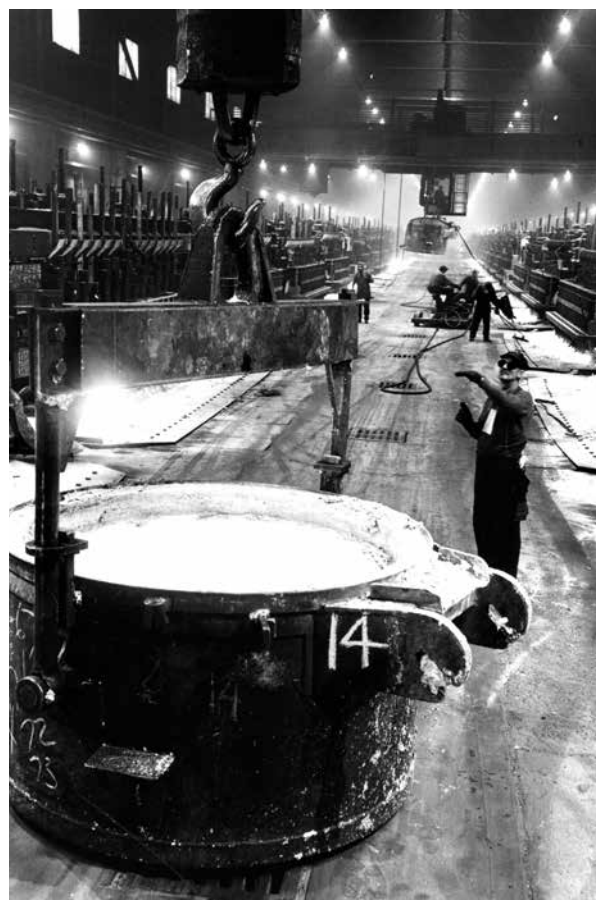
Crucible of molten aluminum ready for casting. Photo courtesy of Rio Tinto.
